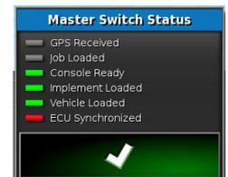
The Master Switch does not switch the spreader in or out of work.
